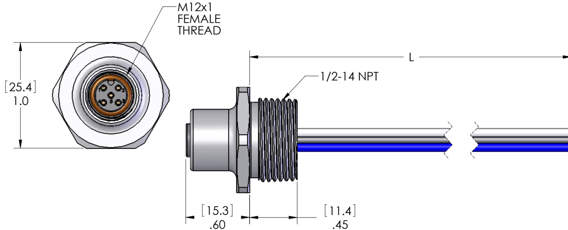
AN O-RING AND LOCKNUT ARE INCLUDED ON LENGTHS OF 19" AND LONGER
