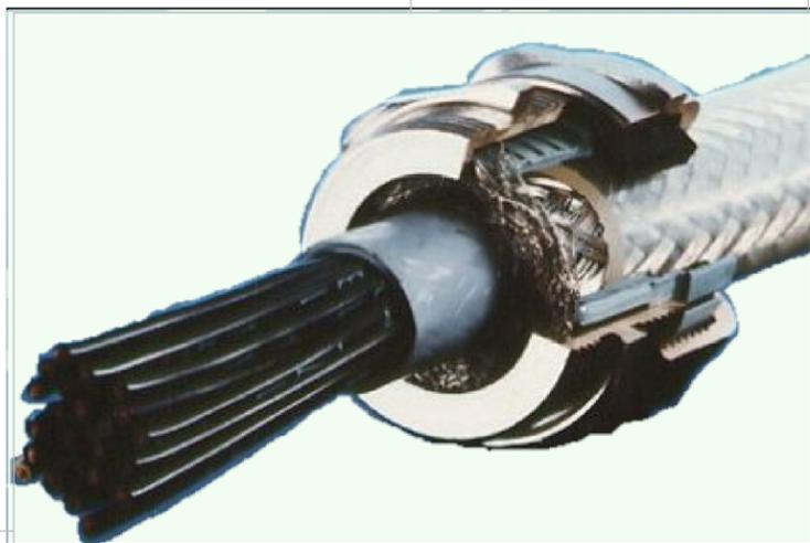
This is a shielding cable gland. For cables with a shield, the shield needs to be folded slightly around the gray plastic insert to allow the shield to be pinched between the gray plastic insert and the bottom of the gland.
