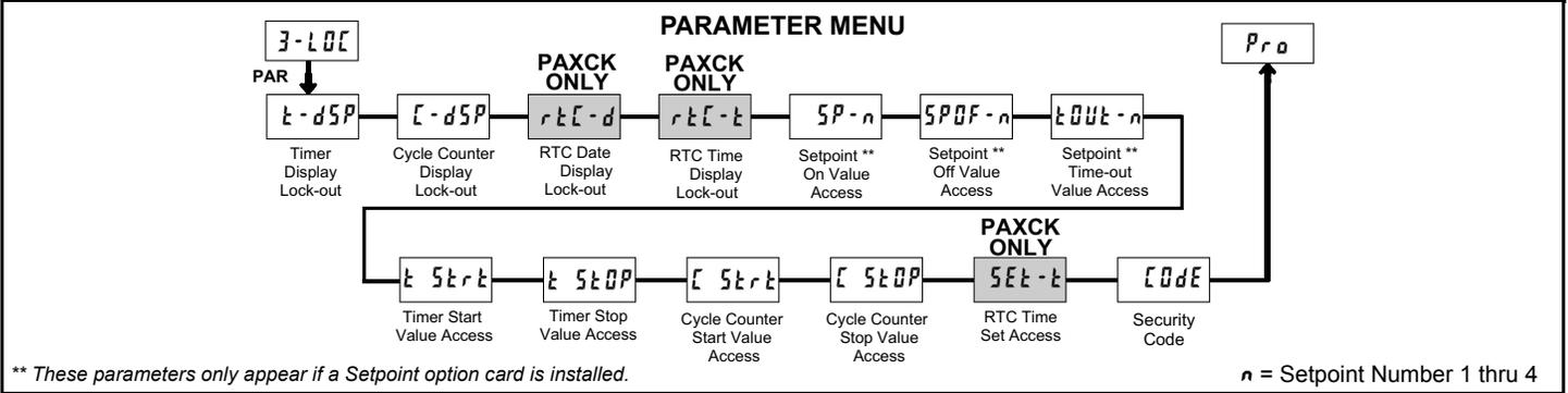
Module 3 is the programming module for setting the Display Lock-out Parameters and the "Quick Programming Mode" Value Access Parameters. In the Quick Programming mode, after the PROGRAM LOCKOUT PARAMETERS and before the Security Code (CODE), a Display Intensity Level (d-LEU) parameter is available when the security code is non-zero. It allows the display intensity to be set to 1 of 16 levels (0-15).
