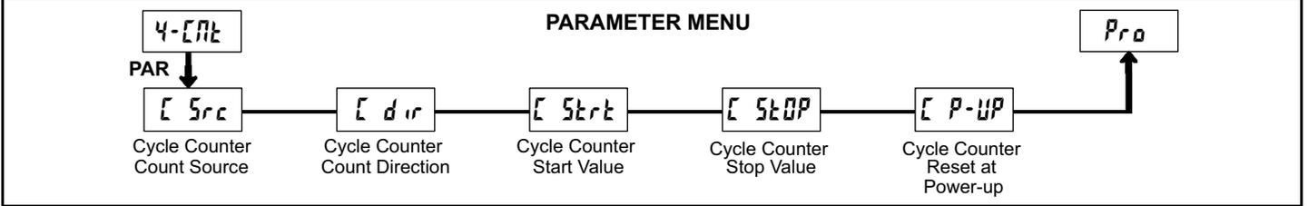
Module 4 is the programming module for the Cycle Counter Parameters. In the Display Mode, the CNT annunciator indicates the Cycle Counter display is currently being shown. An **EXCHANGE PARAMETER LISTS** feature, which includes the Cycle Counter Start and Stop Values, is explained in Module 2.
