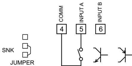
**Switch or Isolated Transistor; Current Source**
