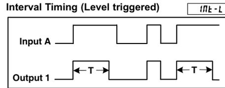
The input signal must be wired to both the Input A and User Input 1 terminals. The Timer Input plug jumper and the User Input plug jumper must both be set to the same position (either both SNK or both SRC).
