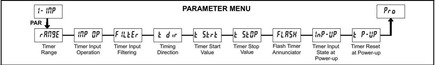
Module 1 is the programming module for the Timer Input Parameters. In the Display Mode, the TMR annunciator indicates the Timer display is currently being shown. An **EXCHANGE PARAMETER LISTS** feature, which includes the Timer Start and Timer Stop Values, is explained in Module 2.
