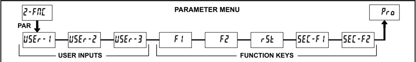
Module 2 is the programming module for the rear terminal User Inputs and front panel Function Keys.
