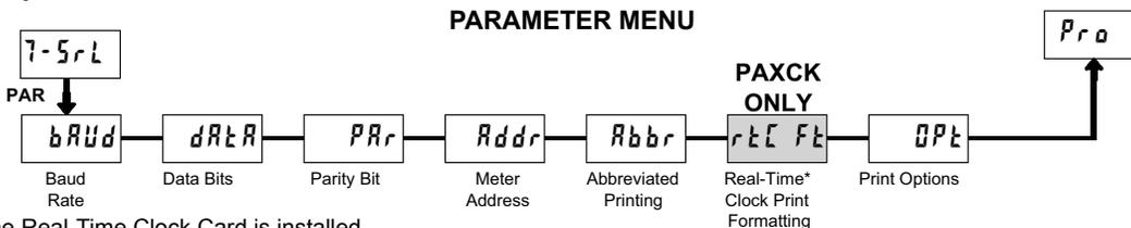
\* Only appears if the Real-Time Clock Card is installed.
