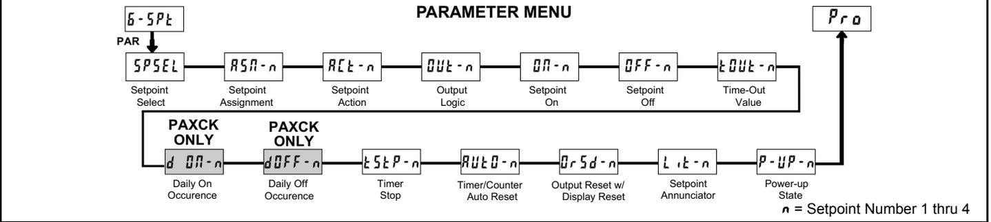
Module 6 is the programming module for the Setpoint (Alarm) Output Parameters. This programming module can only be accessed if a Setpoint card is installed. Depending on the card installed, there will be two or four Setpoint outputs available. The Setpoint Assignment and Setpoint Action parameters determine the applicable Setpoint features, and dictate which subsequent parameters will appear for the Setpoint being programmed.
