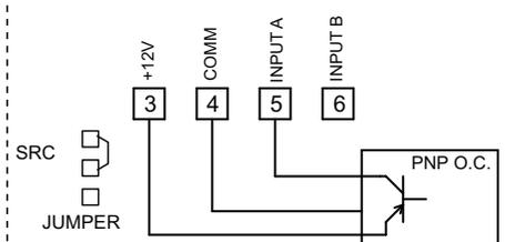
**Switch or Isolated Transistor; Current Sink**
