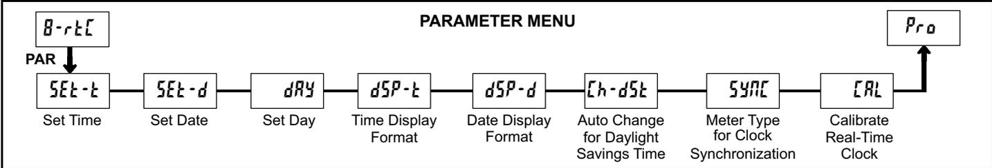
Module 8 is the programming module for the Real-Time Clock (RTC) Date and Time Parameters. In the Display Mode, the DAT annunciator indicates the RTC Date is currently being shown. The RTC Time display is shown with no annunciator. This programming module can only be accessed if a Real-Time Clock card is installed.
