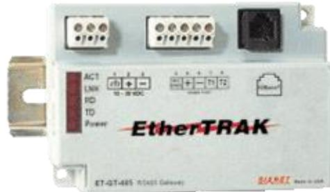
Ethernet to Serial Converters for Modbus, Red lion and other protocols
