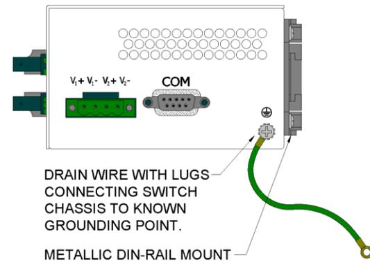
Note: Ensure the power supply is grounded properly before applying power to the grounded switch. This may be verified by using a voltmeter to determine that there is no voltage difference between the power supply's negative output terminal and the chassis grounding point of the switch.
