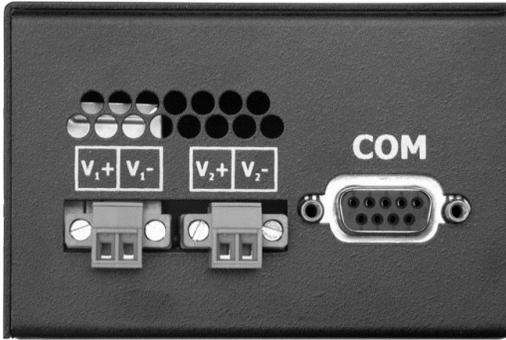
Unscrew & Remove the DC Voltage Input Plug(s) from the side header
