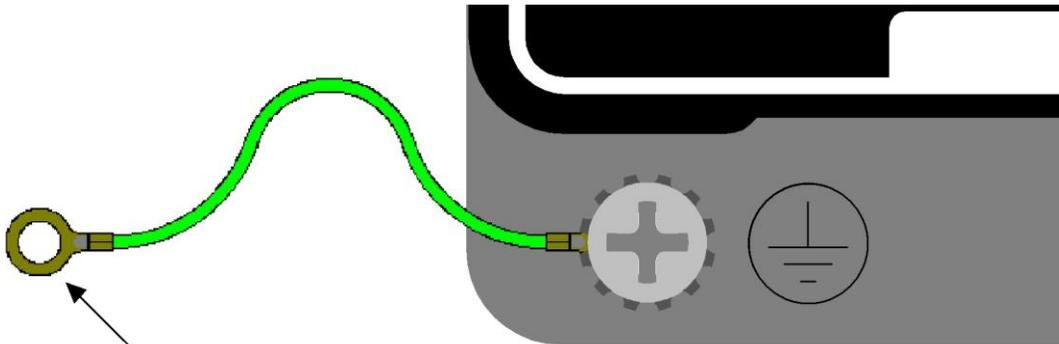
Drain wire with lug connecting switch chassis to known grounding point.
