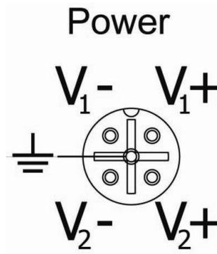
The M12 A coded power connector is keyed, where the mating connection from the power supply can be made only when the male and female ends are lined up properly.
