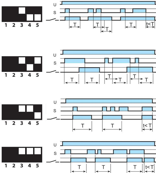
**(BE) Off-delay with control signal**
