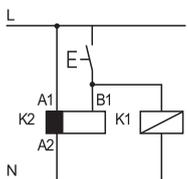
• Possible to control an external load, such as another relay coil or timer, connected to the control signal terminal B1.
