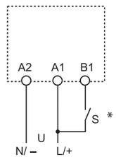
\* With DC supply, positive polarity has to be connected to B1 terminal (according to EN 60204-1).
