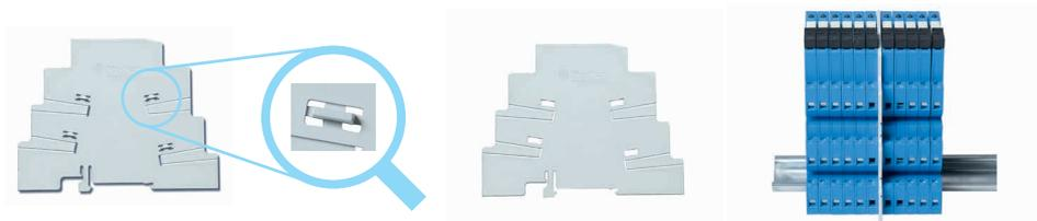
2. Leaving the ribs in place provides 6.2 mm separation. Simply cutting (with scissors) the relevant segment(s) permits the interconnection across the separator of 2 different groups of interface relays, using the standard jumper link.
