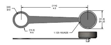
Sealing cap with tether supplied with each unit. NBR tether also acts as gasket for sealing to panel.
