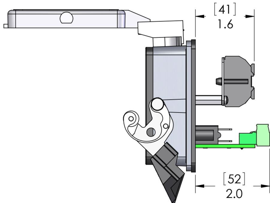
9 PIN D-SUB IS CONNECTED TO A THREE PIN PLUGGABLE TERMINAL BLOCK FOR BLUE HOSE APPLICATION
