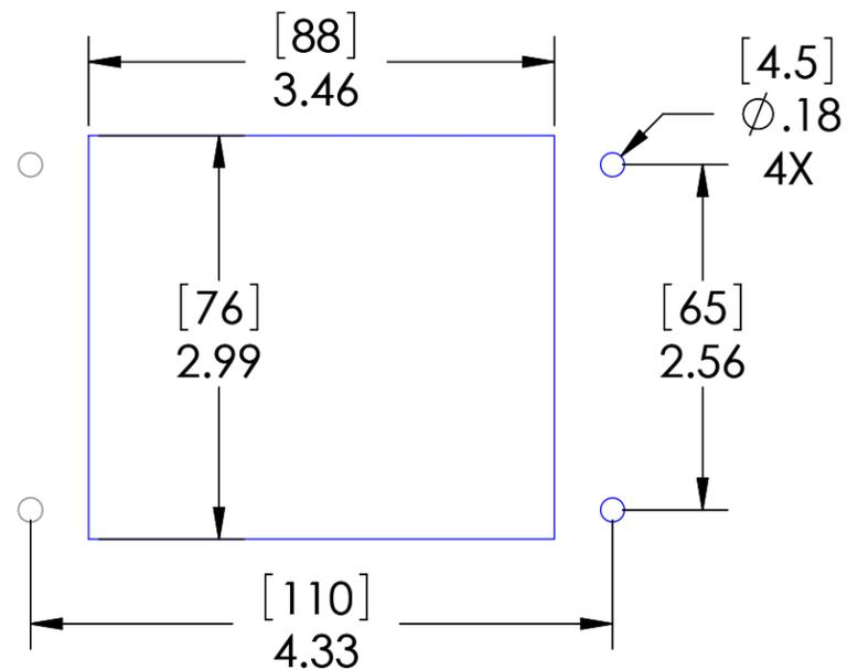
These devices shall be mounted on enclosures having adequate strength and thickness and with adequate spacing provided. Seal rating is based on mounting to a surface that is clean, flat and smooth.
