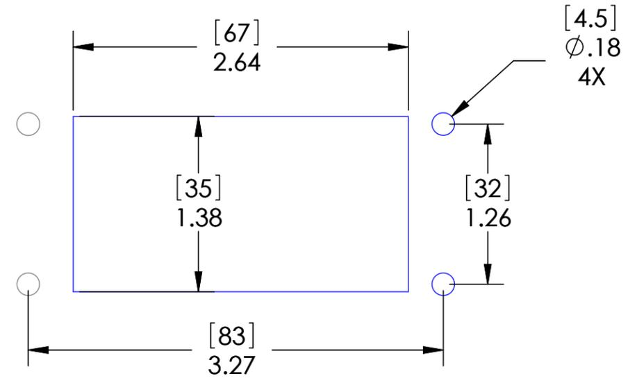
These devices shall be mounted on enclosures having adequate strength and thickness and with adequate spacing provided. Seal rating is based on mounting to a surface that is clean, flat and smooth.
