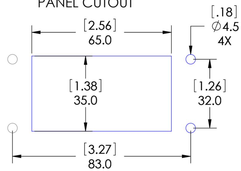
These devices shall be mounted on enclosures having adequate strength and thickness and with adequate spacing provided. Seal rating is based on mounting to a surface that is clean, flat and smooth.
