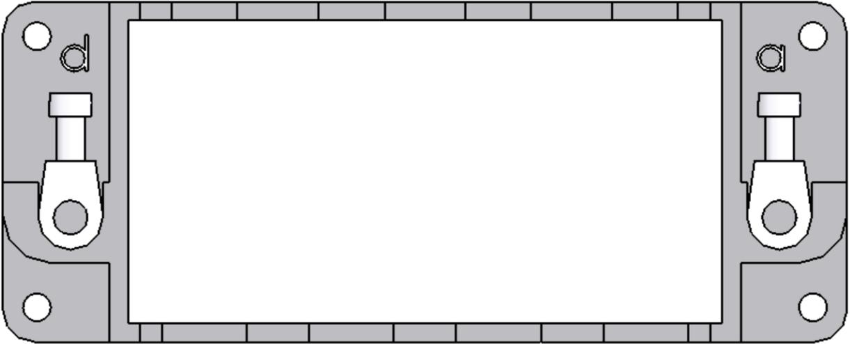
FRAMES CAN BE USED IN EITHER HOODS OR HOUSINGS, FOR CORRECT COUPLING PLEASE USE BOTH FRAME TYPES (ONE WITH UPPER-CASE LETTERS AND THE OTHER WITH LOWER-CASE LETTERS)
