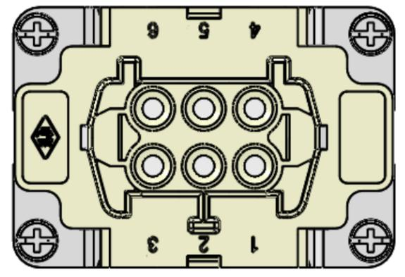
Connection made via spring clamp.
