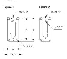
\* For pass-through screws type M3
