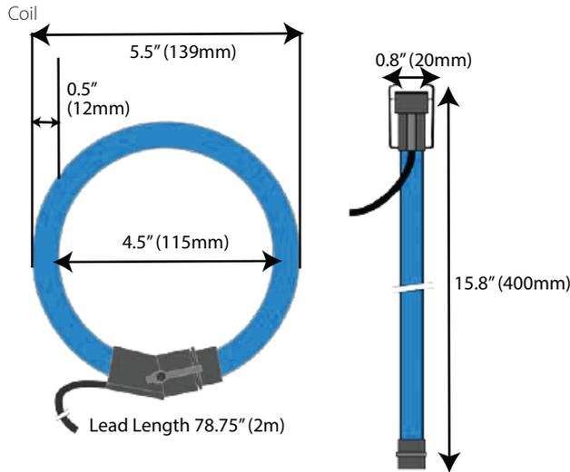
AC Current Transducer Connections
