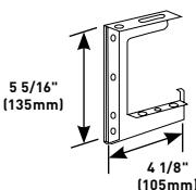
Suspends 3000 Series Raceway from structural ceilings. Designed for use with 3/8" (9.5mm) threaded rod. Hangers should be installed no more than 5' (1.5m) apart along raceway run.
