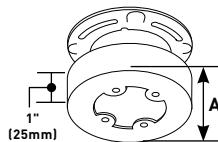
Mounts on 3 1/4" or 4" (83mm or 102mm) conduit boxes or other recessed outlets. Cover accepts devices with mounting screw centers of 2 3/4", 3 1/2" or 4 1/16" (70mm, 89mm, or 103mm). Can be used with 5736 Blank Cover as a pull or junction box.
