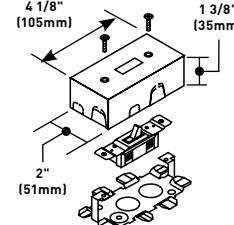
Single pole switch included. Accepts standard single-gang switches including three-way. Cover has twistouts for 500 or 700 Series Raceway on each end and sides. Twistouts on ends of box permit running raceway close to interior trim. Base has 1/2" trade size KO's.
