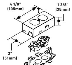
Accommodates 15A (NEMA 5-15R) or 20A (NEMA 5-20R) duplex devices in place of duplex grounding receptacle included. Cover has twistouts for 500 and 700 Series Raceway on each end and sides. Twistouts on ends of box permit running raceway close to interior trim. Base has 1/2" trade size KO's.
