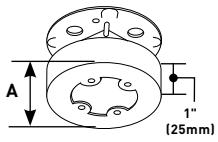
Used to hang fixtures. Cover accepts devices with mounting screw centers of 2 3/4", 3 1/2", and 4 1/16" (70mm, 89mm, and 103mm). Base has four holes for fixture studs, four 1/2" trade size KO's, and raised section for no-bolt fixture-stud. Use as a junction or pull box with 5736 Blank Cover.
