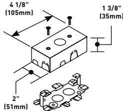
Can be used as tee, cross, pull box, junction box, or blank box. Cover has 1/2" trade size KO and twistouts for 500, and 700 Series Raceway on each end and sides. Twistouts on ends of box permit running raceway close to interior trim. Base has 1/2" trade size KO's.
