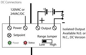
Notes: Terminals are #6 screws. Use up to 14 AWG solid or stranded. Power connections are not polarity sensitive. DC output connections are polarity sensitive.
