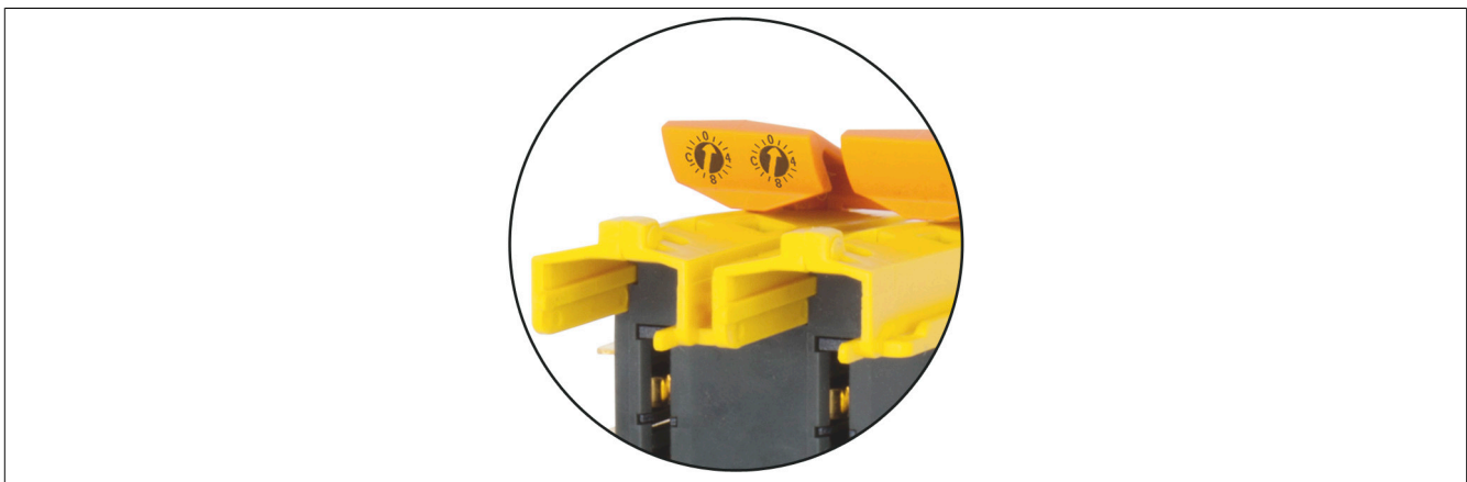
Figure 5: X20BMx6 - Node number switch identification
