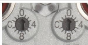
The node number for the POWERLINK node is set using the two number switches.
