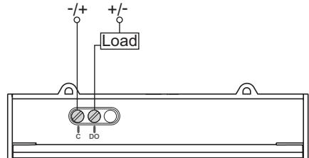
**en** The digital output is polarity-independent.
