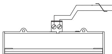
**en** The Lon and M-Bus ports are polarity-independent.
