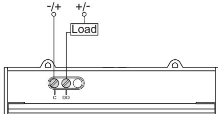
**en** The digital output is polarity-independent.
