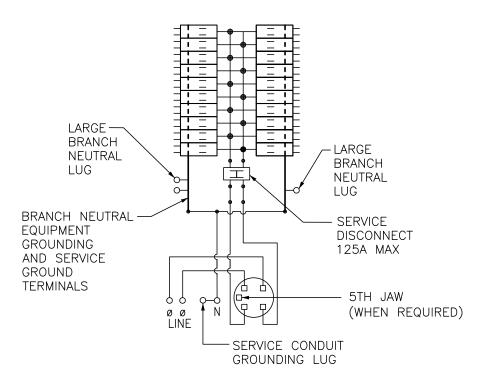
TWO SINGLE POLE, ONE PLUG-ON SPACE TYPE HOMT OR ONE SINGLE POLE, ONE PLUG-ON TYPE HOM OR HOMP. TWO POLE TYPE HOMT, HOM OR HOMA (110A) MAY PLUG ON TWO ADJACENT SPACES.
