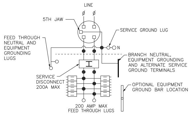
TWO SINGLE POLE, ONE PLUG-ON SPACE TYPE QOT OR ONE SINGLE POLE TYPE QO. TWO POLE TYPE QO, QOA OR QOC (125A MAX) MAY PLUG ON TWO ADJACENT SPACES. TWO POLE QOC (150-200A) MAY PLUG ON FOUR ADJACENT SPACES.
