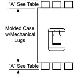
**Table 7.110: Compression Lug Kits for PowerPact™ Circuit Breakers**
