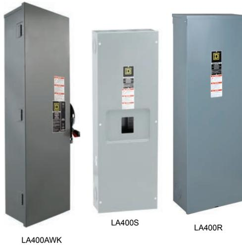
The enclosures for the LA/LH/Q4 thermal-magnetic circuit breakers are UL listed and CSA certified. The enclosures are suitable for service entrance equipment when neutral assembly is installed. The short circuit ratings of these enclosed circuit breakers are equal to the interrupter rating, at the supply voltage marked on the circuit breaker installed.
