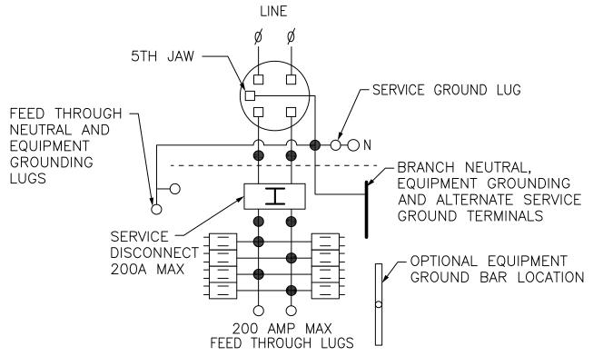
TWO SINGLE POLE, ONE PLUG-ON SPACE TYPE HOMT OR ONE SINGLE POLE TYPE HOM. TWO POLE TYPE HOMT, HOM OR HOMA (125A MAX) MAY PLUG ON TWO ADJACENT SPACES.
