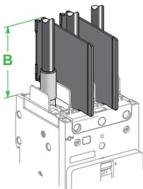
Interphase barriers provide phase to phase isolation at the power-connection points:
