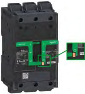
PowerPacT B-frame circuit breakers have an over-center toggle mechanism providing quick-make, quick-break operation. The operating mechanism is also trip-free, which allows tripping even when the circuit breaker handle is held in the “ON” position.
