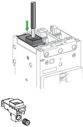
Mechanical lugs suitable for copper and aluminum conductors are available as field-installable kits or factory assembled. (Refer to Connection Accessories, page 107.)
