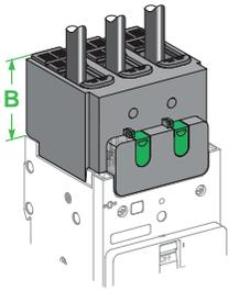
Products can be equipped with long terminal shields. They can be mounted upstream and downstream and are used for protection against direct contact with power circuits. They provide IP40 degree of protection and IK07 mechanical impact protection. The long terminal shield can be mounted after product installation on a plate or DIN rail, and can be removed and put in place even if there are auxiliary wires installed. They are not compatible with EverLink connectors.
