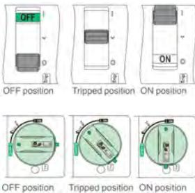
The circuit breaker handle can assume any of three positions: ON, tripped or OFF.
