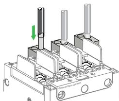
The power distribution connectors (PDCs) can be used for multiple load wire connections on one circuit breaker. Use in place of stand-alone power distribution blocks to save space and time. Field-installable kit includes tin-plated aluminum multi-conductor lug, interphase barriers, and required M6 x 24 mm mounting hardware.
