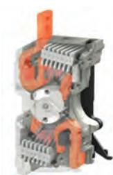
All PowerPacT B-frame circuit breakers are equipped with dual-break rotating contacts that reduce the amount of peak current during a short circuit fault. This reduces the let-through currents and enhances equipment protection.
