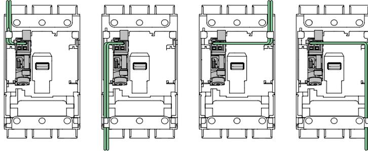
Electrical accessory wire routing can be exited out either of the two load-end corners of the I-Line circuit breaker, under the accessory cover even when using the load-end long terminal shield.
