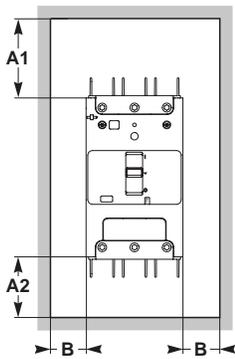
For all types of PowerPacT B-frame circuit breakers that use uninsulated power connections (for example, busbars, spreaders, or uninsulated compression lugs), the minimum clearance distance between the enclosure backplate (grounded metal) and uninsulated power connections is shown below.
