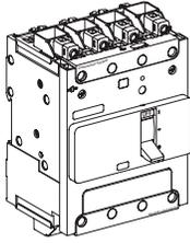
**B-Frame, 4P, 600Y/347 Vac, 250 Vdc, with EverLink™ Connectors, Factory-Sealed Trip Unit**
