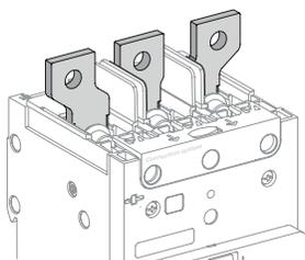
Spreaders can be used to increase the pitch of the circuit breaker from 27 mm (1.063 in.) to 35 mm (1.378 in.). They are delivered with interphase barriers and M8 screws, nuts and washers. The connectors are attached to device terminals equipped with separately provided terminal nut connectors.
