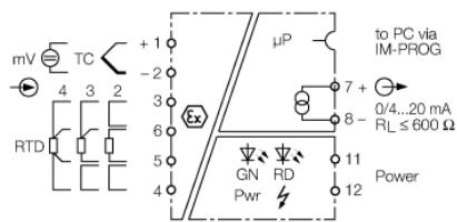
The 1-channel Ex-area temperature measuring amplifier IM34-11EX-CI/K51 is designed to evaluate the temperature-dependent changes of Ni100/Pt100 RTDs, thermocouples types B, E, J, K, L, N, R, S and T or low voltages in a range of -160...+160 mV and to output them as temperature-linear current signals 0/4...20 mA.
