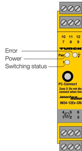
The 1-channel Ex-area temperature measuring amplifier IM34-12EX-CRI is designed to evaluate the temperature-dependent changes of Ni100/Pt100 RTDs, thermocouples types B, E, J, K, L, N, R, S and T or low voltages in a range of -160...+160 mV and to output them as temperature-linear current signals 0/4...20 mA.
