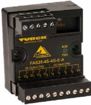
This module provides one connector with four PNP inputs and four PNP outputs each for connection to AS-interface®. The wiring is simple screw terminals to support multiple I/O configurations.
