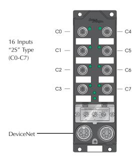
This  $busstop^{\circledast}$  station takes in up to sixteen discrete three-wire inputs or eight discrete four-wire input points per node. There are two inputs per connector-one on pin four and one on pin two.
