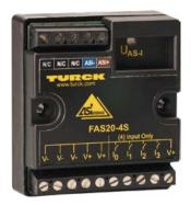
This module has four inputs. Inputs are protected against short-circuit as a group. If any input has shorted, the entire group of inputs are disconnected from bus power.
