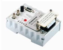
The optocoupler OC11Ex/2G.2 converts the PROFIBUS-DP signals on copper cables into optical signals. The bus signals can therefore be transmitted from the safe area to the Ex area over long distances without potential or interference. When using fiber-optic cables, the maximum baud range is 2500 m for OM1 (62.5/125- $\mu$ m) cables and 1500 m for OM2 (50/125- $\mu$ m) cables.
