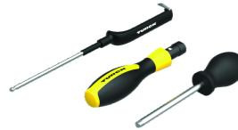
Adjustable torque driver to connect to the 13mm hex. Compatible with redesigned M12 cordsets, M12 Power, and M12 X-code. NOT Compatible with legacy M12 cordsets. Includes (1) adjustable torque driver, (1) adjustment tool, and (1) 13mm forklift bit.
