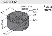
Positioning element for encoder RI-QR20, for Ø 6.35 mm shafts
