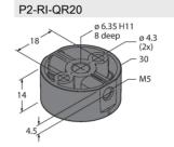
Positioning element for encoder RI-QR20, for Ø 6.35 mm shafts
