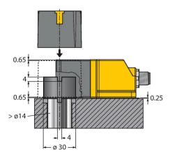
Ri-DSU35 for mounting on rotary actuators The Ri-DSU35 angle sensor and the well-established Ni4-DSU35 inductive dual sensor are identical in construction. The user also profits from the enormous mounting flexibility of the device. The sensor can be mounted on all standard rotary actuators with a shaft diameter of max. 14 mm thanks to an extensive range of available accessories. For larger shaft diameters use the BTS-DSU35-Z02 accessories.
