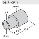
1590814 Spacer sleeves for rear mounting of RI-QR14, 2 pcs. per bag
