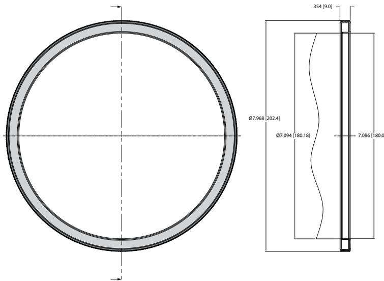
Magnetic Ring (press fit) for pulse rate: 700, 2240, 2800, 7000
