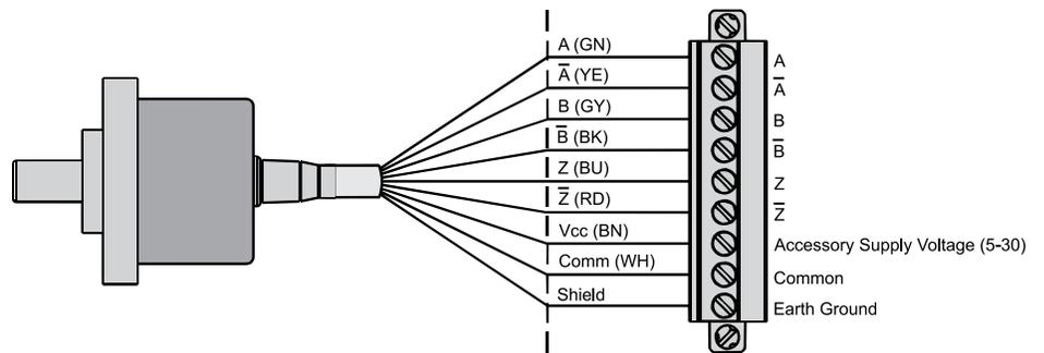
For general industrial environments where there are no large motor or drives present, the standard M12 Eurofast® cordset with non-twisted pair conductors will suffice. In heavy industrial environments, or when used on AC vector motors, M12 Eurofast cordsets with twisted pairs should be used.
