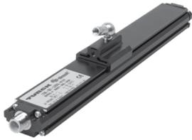
EZ-track LDT's profile style probes use magnetostrictive technology by applying a mechanical strain pulse to a magnetostrictive waveguide that runs the length of the sensor. When the strain pulse encounters a magnetic field produced by the slide or floating magnet assembly, a current pulse is produced that is picked up by the electronic circuitry. A high
