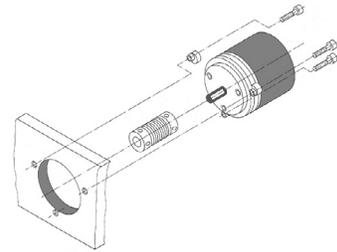
Mounting with assembly bell, fastening eccentrics and coupling (to prevent shaft overload and to insulate the encoder thermally and electrically).
