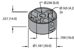
Positioning element, operating at a distance of 0-5 mm to the sensor surface. Nominal distance is 1 mm.
