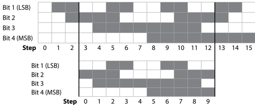
**Reversion of the gray code:** The code values increase when the shaft is turning clockwise. If the most significant bit (MSB) is inverted, the code values decrease when the shaft is turning clockwise.
