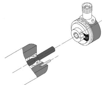
Mounting of a hollow shaft encoder with extended torque stop and long pin.
