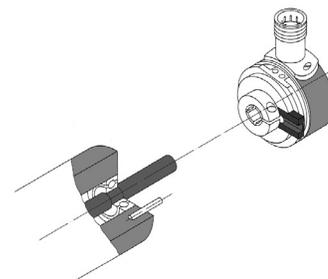
Mounting of a hollow shaft encoder with a flex coupling.
