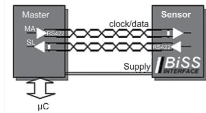
With every data cycle the master learns and compensates for the signal transit times, thus enabling high clock rates up to 10M bit/s even with cable lengths of 100 m. Varying cable conditions, for example due to drag movement, are corrected. The synchronization accuracy between several encoders on a number of axes is less than one microsecond; moreover the master keeps the signal transit times that have been experienced transparent for the controller and thus enables a further optimization.
