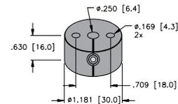
Positioning element, operating at a distance of 0-5 mm to the sensor surface. Nominal distance is 1.5 mm.
