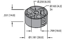
Positioning element, operating at a distance of 0-5 mm to the sensor surface. Nominal distance is 1 mm.
