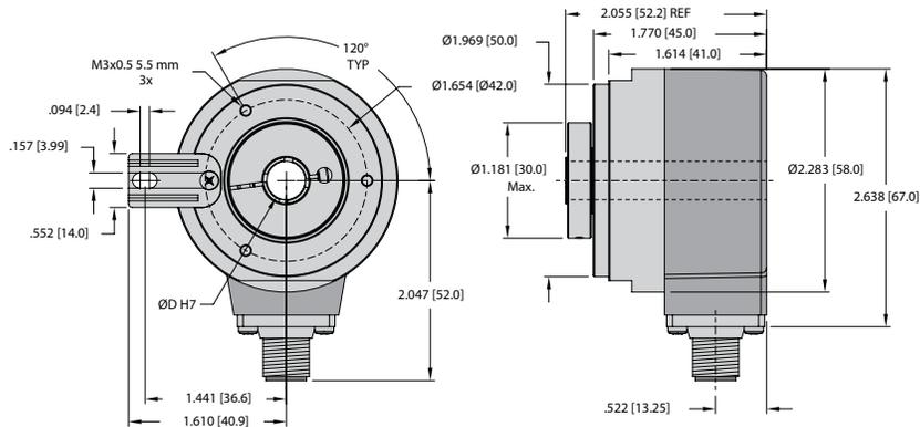
1) Torque stop recommendation: cylindrical pin DIN 7, Ø0.16 [4.0]
