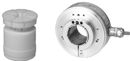
The RI-43 encoder is used for AC vector motor and general industrial applications. For AC vector motor applications, the encoder should be electrically isolated from the motor chassis to minimize encoder bearing currents and ground noise. An isolation insert for the hollow shaft is provided with the encoder by specifying N42 in the "special insert option" decode. **When ordering isolation inserts separately, choose option 38 with a bore diameter of 38 mm.**
