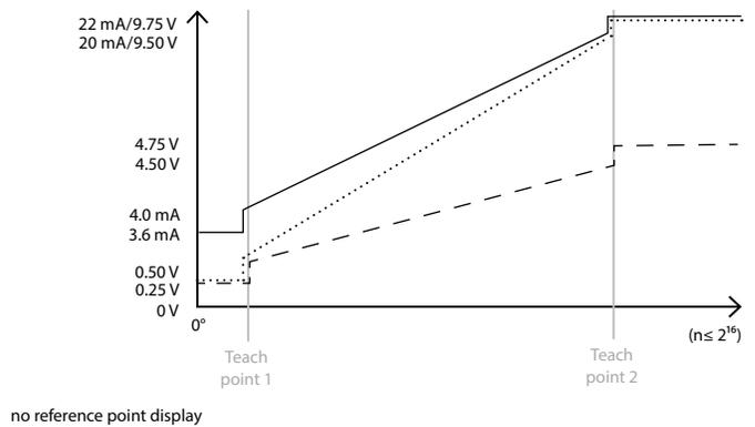
**Note:** Factory-set measuring range:  $2^4$  revolutions with roll-over
