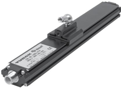
The Q21D is a non-contact LDT with a digital output. This transducer utilizes magnetostrictive technology to give absolute position that is repeatable to .006% of the active sensing distance. It also has the same auto-tuning capability that the other profile series transducers offer, so that it can adjust its signal strength to various magnets.
