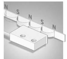
The system is not affected by dust, shavings or humidity and is resistant to many liquids and to oil. Assembly is easy; the magnetic band just has to be glued into place. There are no problems for calibration. The distance between the sensor and the magnetic band can be up to two mm. Repeat accuracy is very high.
