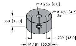
Positioning element, operating at a distance of 0-5 mm to the sensor surface. Nominal distance is 1.5 mm.
