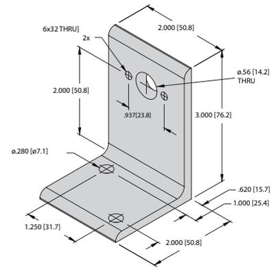
**MB-R10:** Part number includes mounting bracket **LB-R10** and rod support bracket **RB-R10**.
