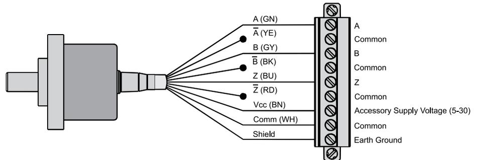
Complements (A not, B not, Z not) should never be tied to common or to each other. The unused wires should be tied back and insulated to prevent them from touching Vcc, common or any other signal wires or driver damage can occur.
