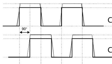
Signals of an older encoder without aging compensation:
