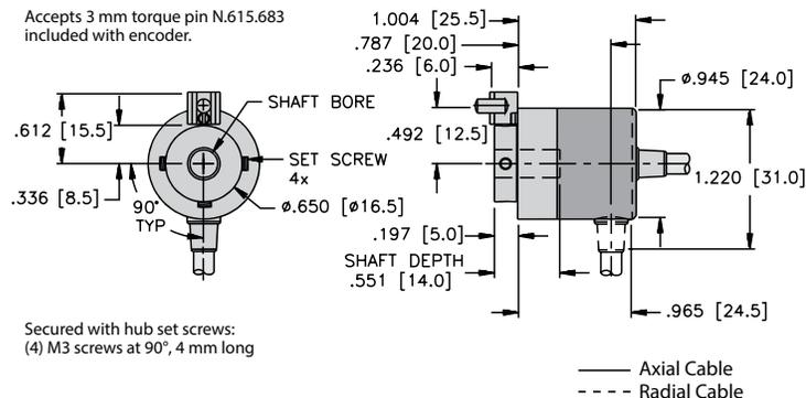
Secured with hub set screws:
