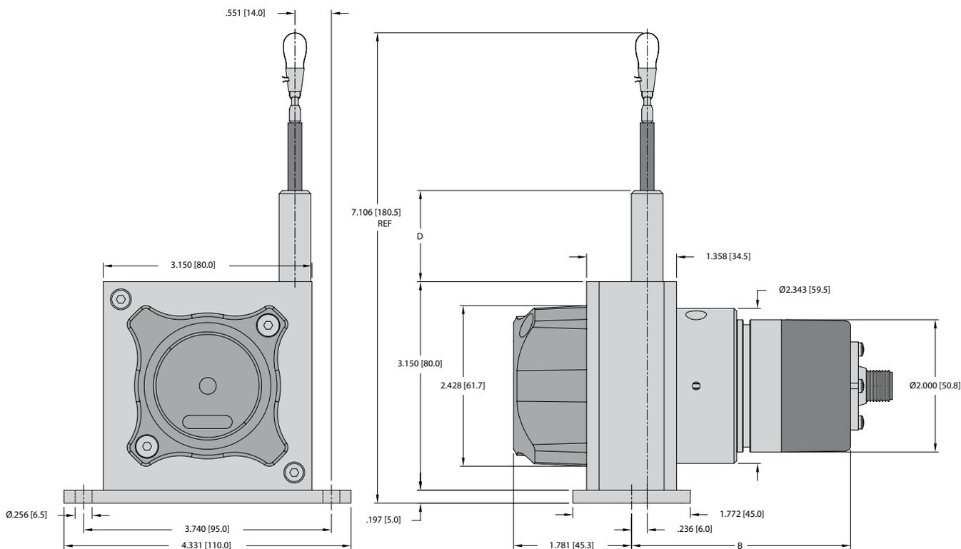
Dimension D depends on the measuring range of the draw wire
