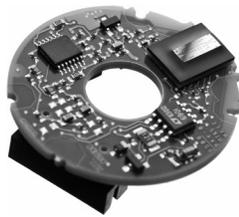
OptoASIC and Intelligent Scan Technology (IST) is the latest development in Absolute encoder technology. The development of an OptoASIC with Intelligent Scan Technology enabled Turck to build the first optical multiturn encoder without gears or magnetic sensors.
