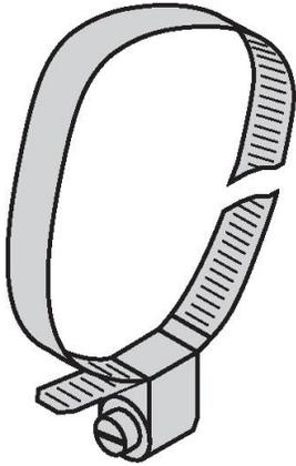
Clip collar for mounting brackets for magnetic field sensors on round cylinders; cylinder diameter: 28... 39 mm; other lengths are available under designations ASB-1 to ASB-9
