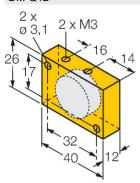
Actuator, rectangular, plastic, attainable switching distance 58 mm on BIM-(E)M12 magnetic field sensors or 49 mm on BIM-EG08 magnetic field sensors; for Q25L linear position sensors: recommended distance between the sensor and magnet: 3...5 mm
