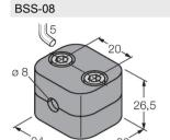
Mounting clamp for smooth and threaded barrel sensors; material: Polypropylene
