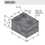
Mounting clamp for smooth barrel sensors; mounting block material: Anodized aluminum
