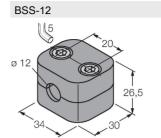
Mounting clamp for smooth and threaded barrel sensors; material: Polypropylene
