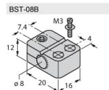
6947210 Mounting clamp for threaded barrel sensors, with dead-stop; material:
