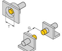
All non-flush mountable cylindrical uprox+ sensors can be screwed to the upper edge of the barrel. Safe operation of the  $\varnothing$  6.5 mm version is guaranteed with reduced switching distance of max. 30 %.
