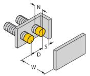
All non-flush mountable uprox®+ threaded barrel sensors can be screwed to the upper edge of the barrel. In this mounting position, the sensor operates safely with a 20 % reduced switching distance.
