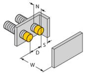
All non-flush mountable uprox®+ threaded barrel sensors can be screwed to the upper edge of the barrel. In this mounting position, the sensor operates safely with a 20 % reduced switching distance.
