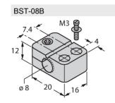
6947210 Mounting clamp for threaded barrel sensors, with dead-stop; material: PA6
