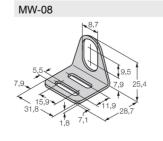
6945008 Mounting bracket for threaded barrel sensors; material: Stainless steel A2 1.4301 (AISI 304)
